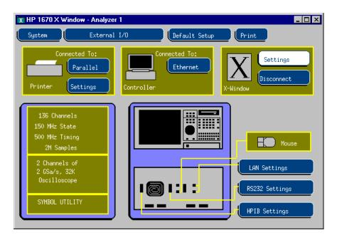
A window that looks like the logic analyzer display will appear on your workstation and you will be able to control the analyzer from the workstation by using the mouse (touch-screen is not available for remote control).
